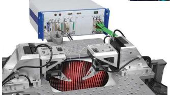
A Silicon Photonics test and alignment system
