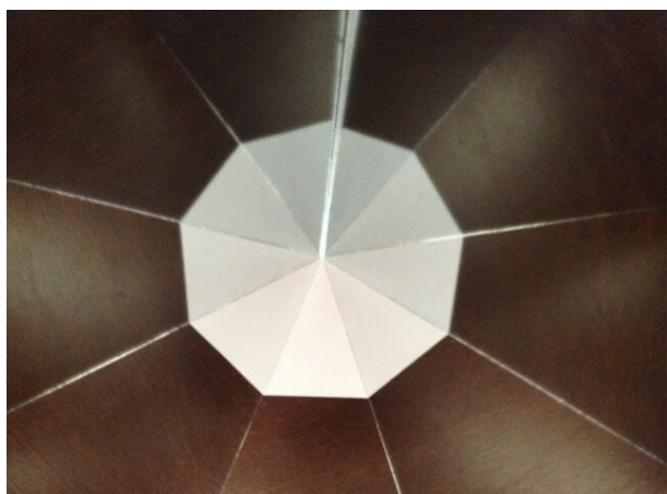
Nanogan - Angle between the mirrors is 40 degrees.
