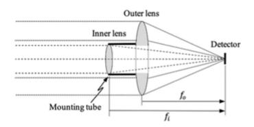
and detailed using raytrace methods by Phenis et al. [Proc. of SPIE, 11125(111250J), (2019)]. The motivation of the lens is to reduce the return signal with targets (objects) relatively near and boost the signal at far range targets by combining lens elements in parallel rather than in series. Using the techniques provided, a designer can develop a lens requiring a detector with less dynamic range and/or extend the far range limit while maintaining the minimum target
